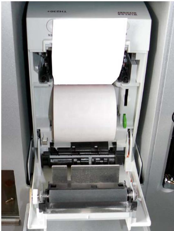
Hold down the paper and close the printer cover. Press on the middle of the cover until it audibly and distinctly locks into place.
