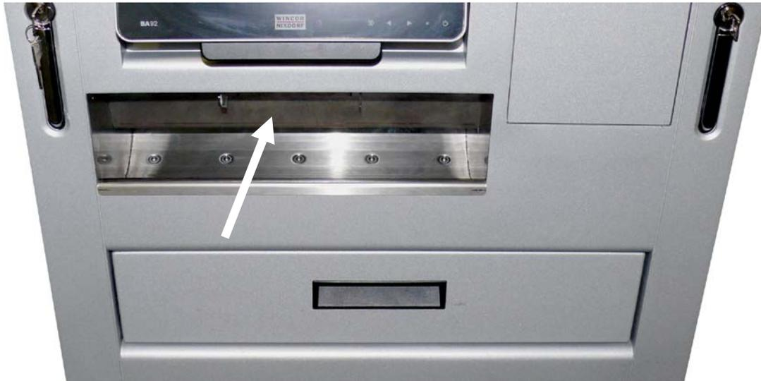
Clean the return compartment and remove foreign objects from the return compartment.
