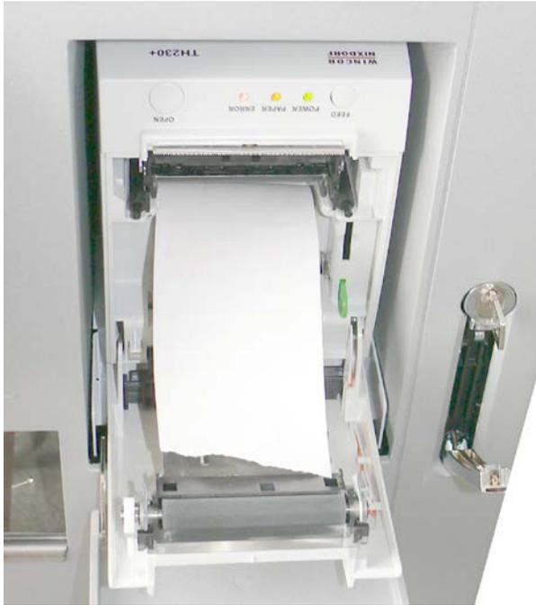
Lay the unwinded paper over the front edge of the printer.
